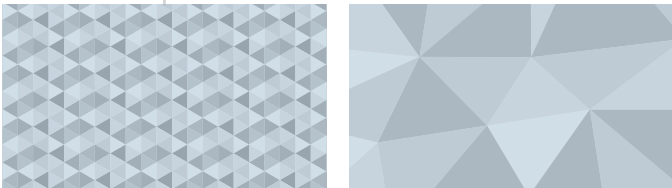
with an Irinox blast chiller formation of microcrystals | formation of macrocrystals without a blast chiller
